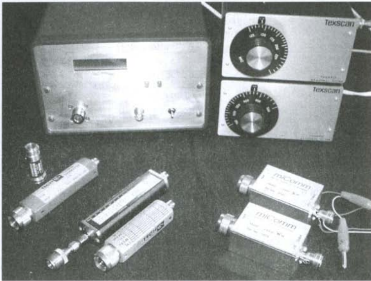
Fig. 11: SPANFI, variable octave bandpass filters, miComm LNAs (as D.U.T.s), different noise generators and fixed attenuator.
